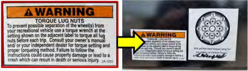
Lug nut torque pattern and warning label
